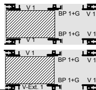
1 Top: for backplane Bottom: for backplane/ front horizontal rail with 10 mm extension
